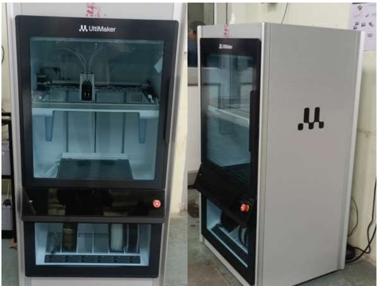
3D Printing - Plastic (Ultimotor Factor 4, FDM)
